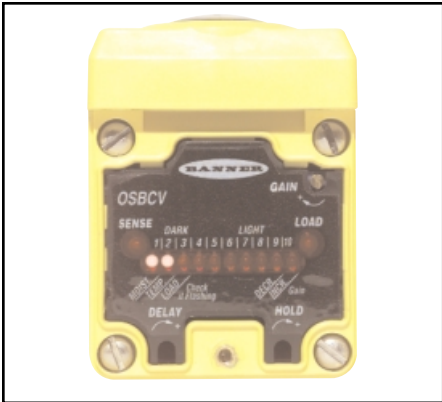
Figure 8. Dark condition example: D.A.T.A. system LEDs #1 and #2 lit.
