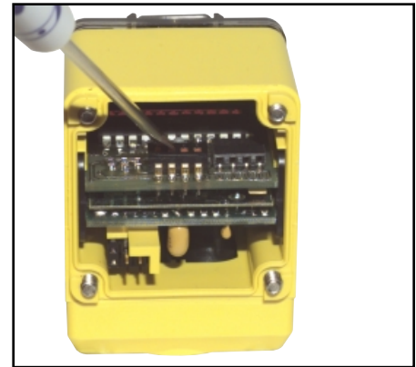
Figure 5. OMNI-BEAM program switches
