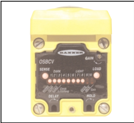
Figure 9. Light condition example: D.A.T.A. system LEDs #1 through #8 lit.
