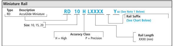
$\underline{\textbf{Note 1}} \ \textbf{-} \ \textbf{Y=Distance from end of rail to center of 1st mounting hole}$
